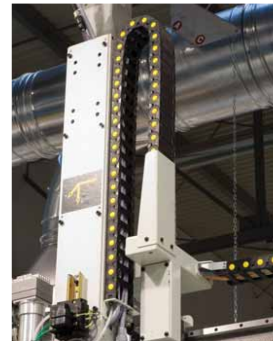
Catena in nylon in corsa verticale
